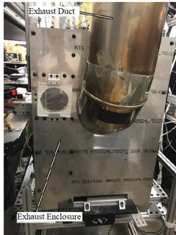
Figure 46: COAL lab initial exhaust enclosure and optical access point [33]
