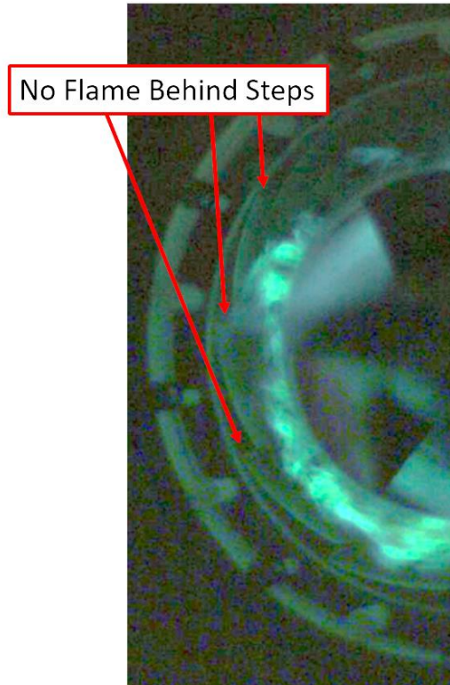
Figure 98: Circumferential cavity combustion 0.273 seconds prior to flameout
