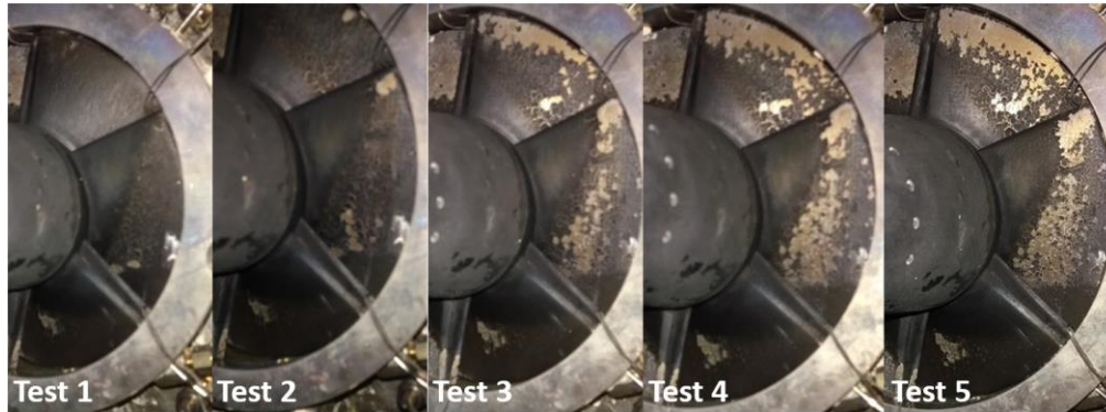
Figure 55: Paint condition post test for five consecutive trials
